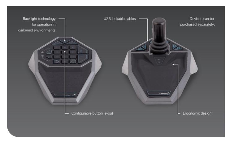
Users may easily map operational commands to hot-keys and reconfigure button layouts of both the EX300 Keypad and Joystick. These features allow individual users to tailor the device to their personal or workstation requirements for efficient access to the appropriate functionality at the right time.
